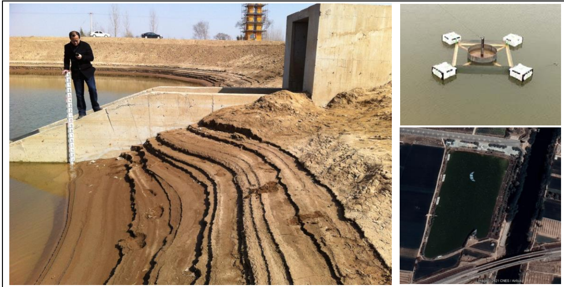
Figure 23: Infiltration basin in Guantao County with water depth gauge (left) and floating evaporation pan (upper right) to measure evaporative losses. A satellite image (bottom right) shows the extent of the infiltration pond, which is called “Moon Lake”.
