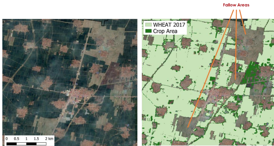
Figure 60: Identification of fallowed wheat areas by comparison of images from two consecutive years.
