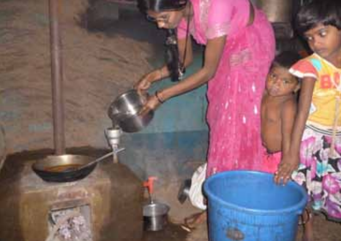
WOTR's hot water chullah
