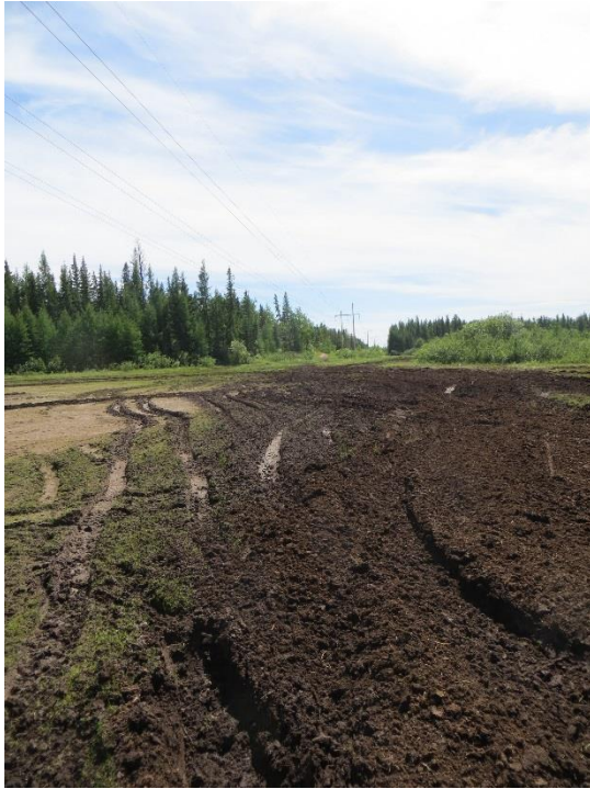
Figure 16. Examples of soil compaction and rutting from off road vehicles along powerline right-of-way near Grande Prairie, Alberta (left) and from highway vehicles on access road near Wabasca, Alberta (right).
