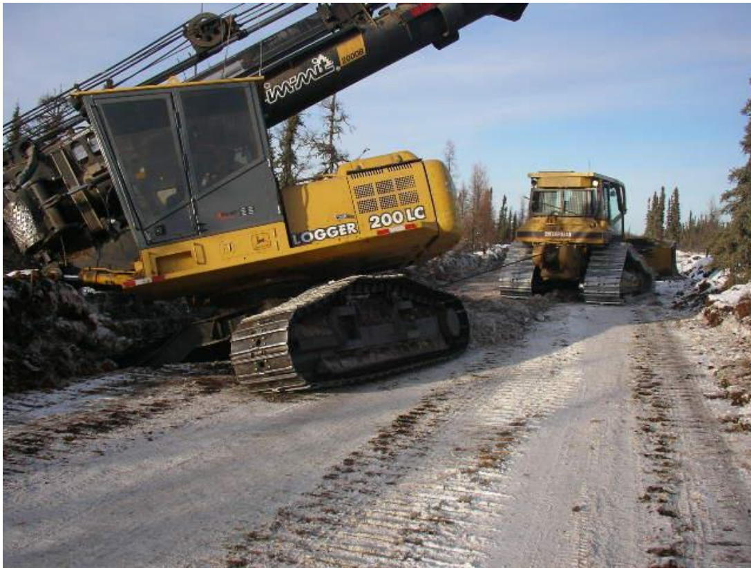
Figure 13. Example of equipment submerged in a peatland. Understanding wetland type can provide information about potential peat depth and subsurface water flow, important considerations for making safe decisions when operating in and around wetlands. Photo credit Millar Western Forest Products Ltd.
