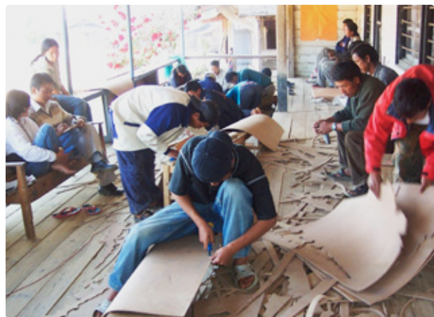
Figure 31. Participants cutting out layers of EVA/PE foam sheets to manufacture a 3D model in Nepal. Image courtesy Ms. Apoorva© ENRAP/IDRC
