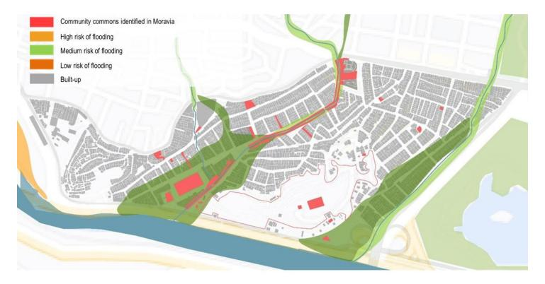
In Moravia, the current high vulnerability to flooding – that tends to increase in a scenario of more frequent torrential rains-is connected to the informal occupation of the creeks and blockage of natural drainage systems.
