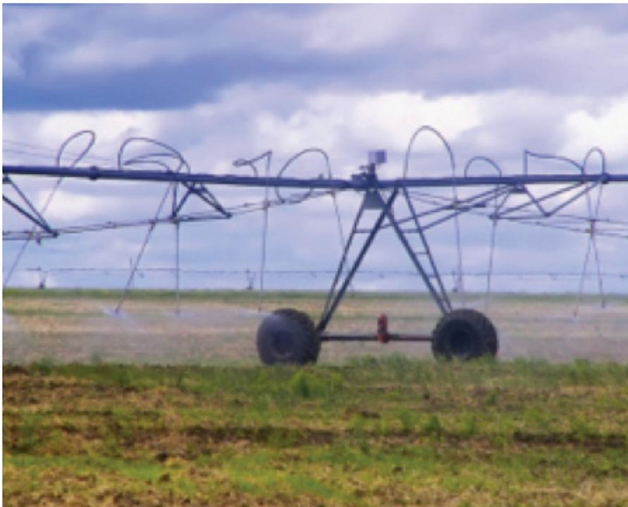
**Irrigation machineries with spaying nozzles for near-surface irrigation**
