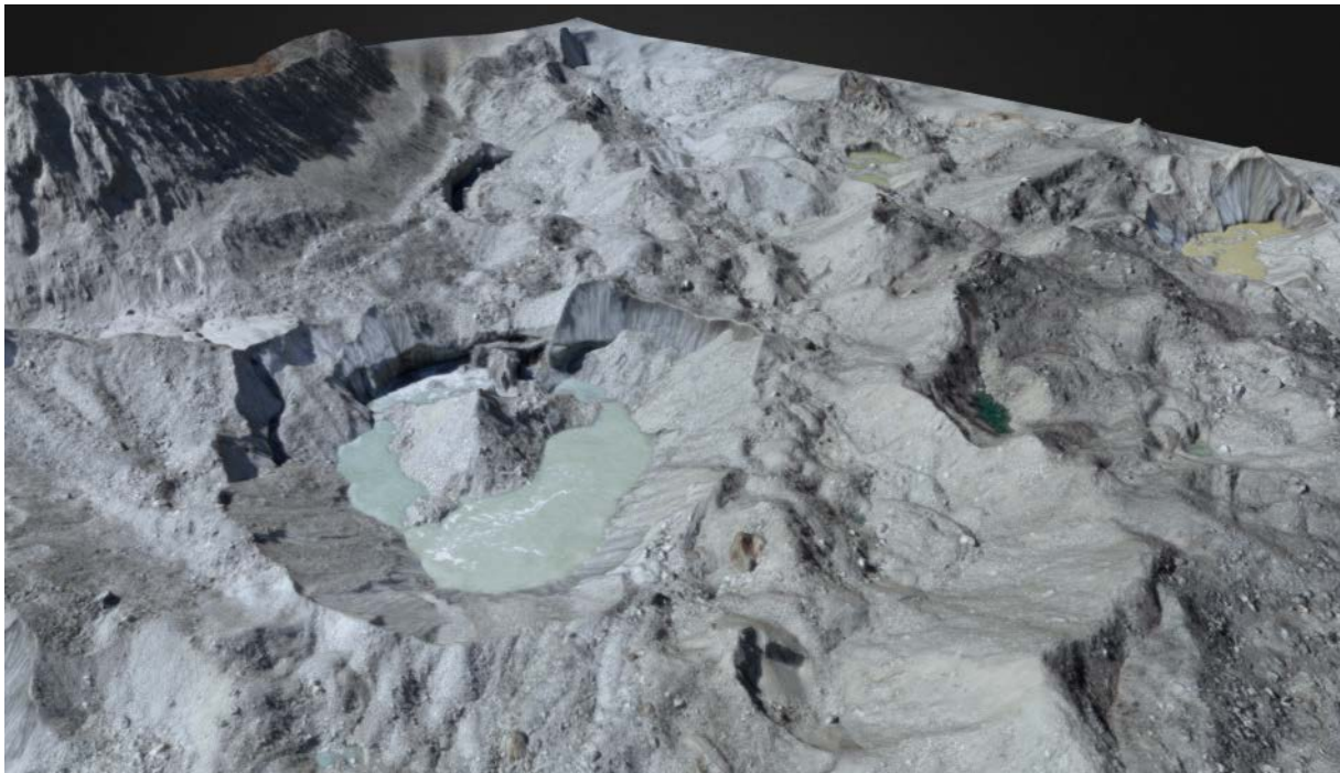
Figure9: 3D model constructed in SketchFab of the Langtang glacier based on UAV data.
