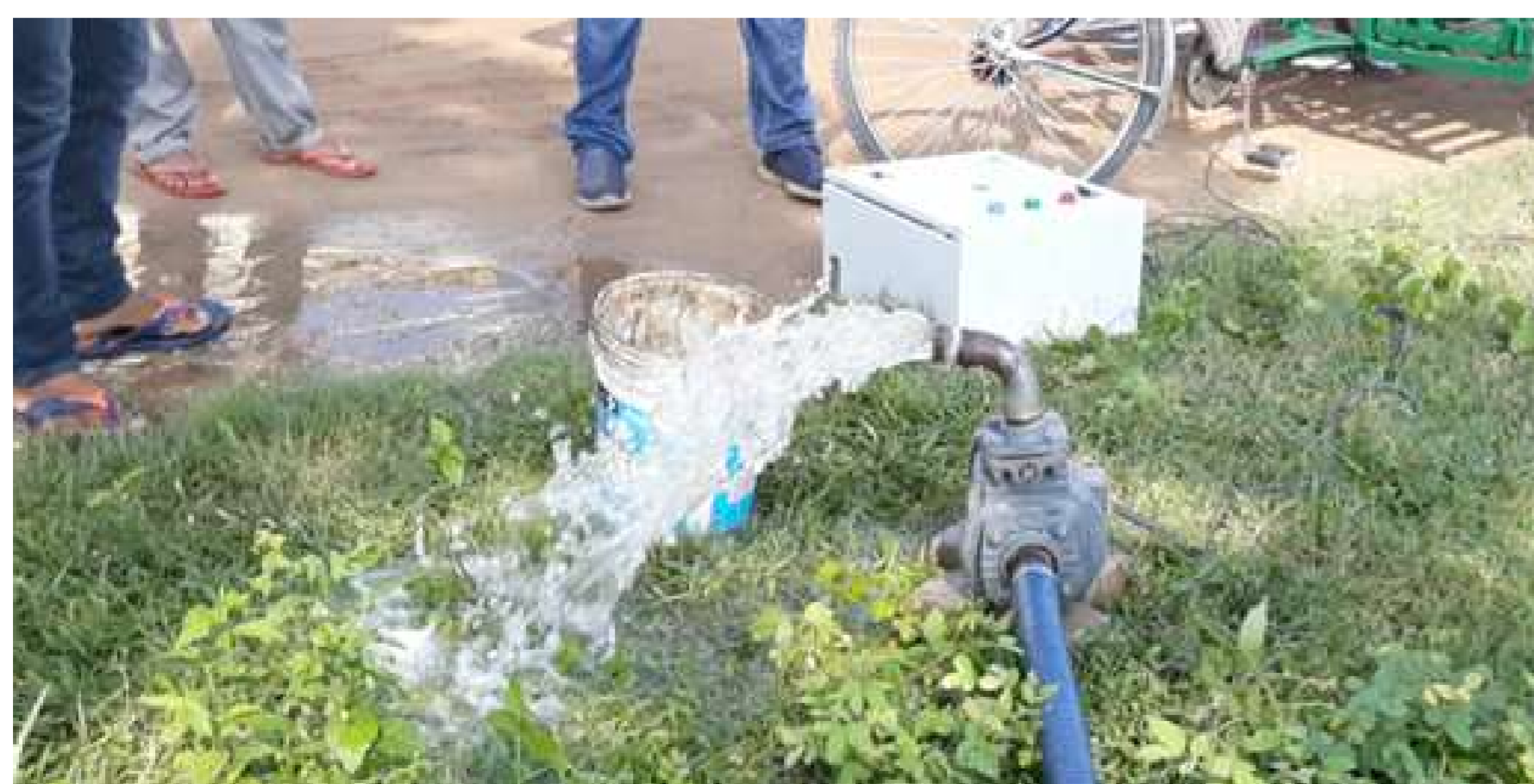
Solar mobile pump and usage
